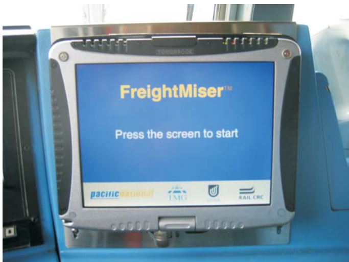
The FREIGHTMISER on-board advice unit installed on a locomotive and ready to provide energy-optimal driving advice.
